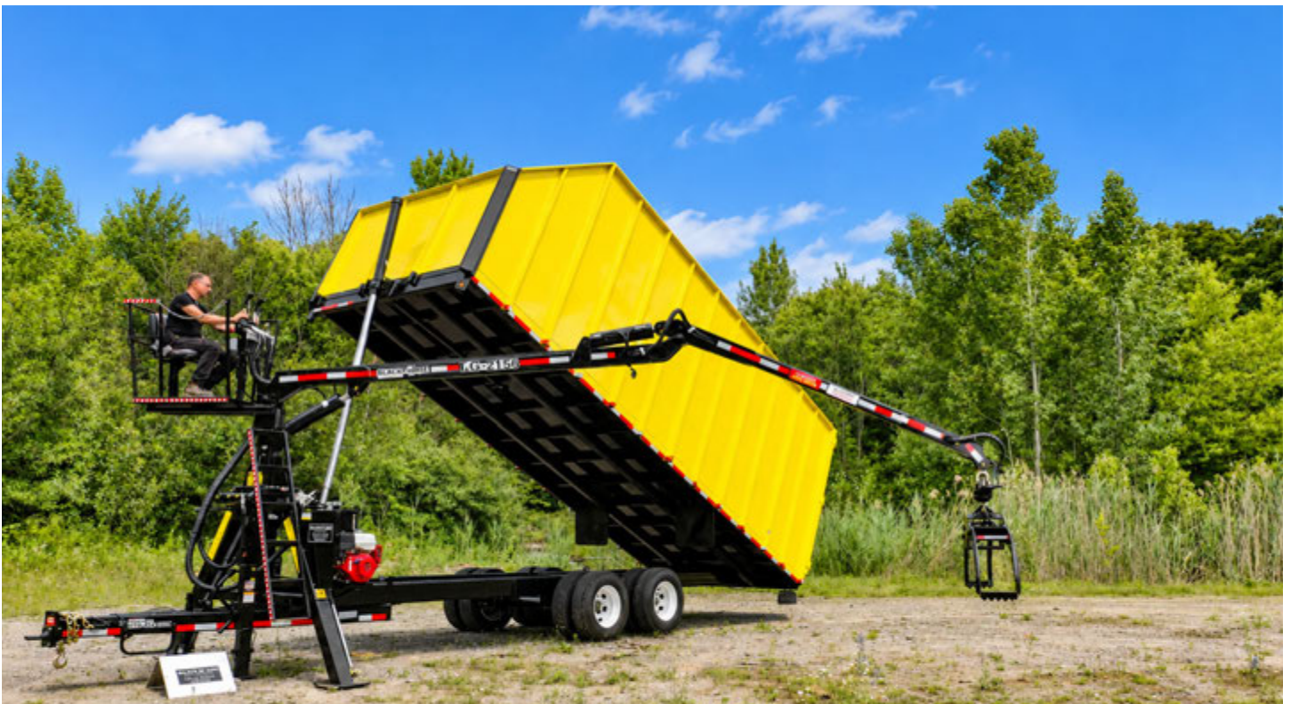
Model LTD824-30K with optional 6' solid steel side extensions, LG-2356 log loader with operators platform and Honda power pack.
