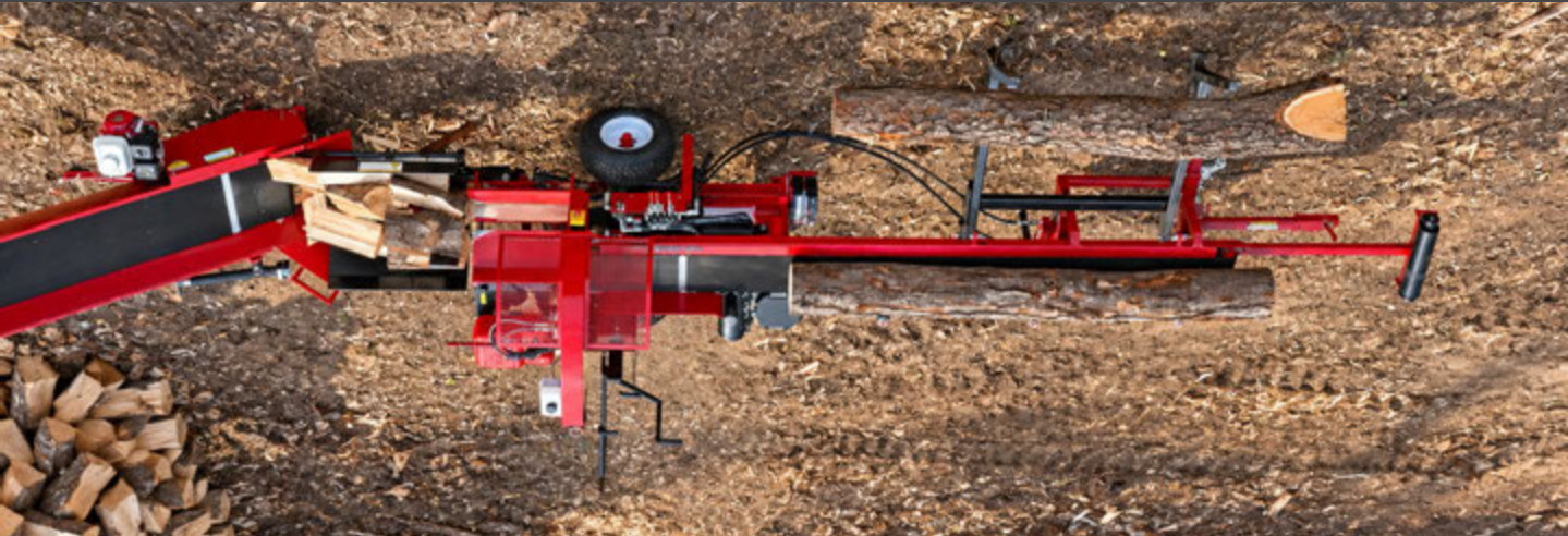
2000B-XL Processor is shown with optional hydraulic log loader and conveyor.
