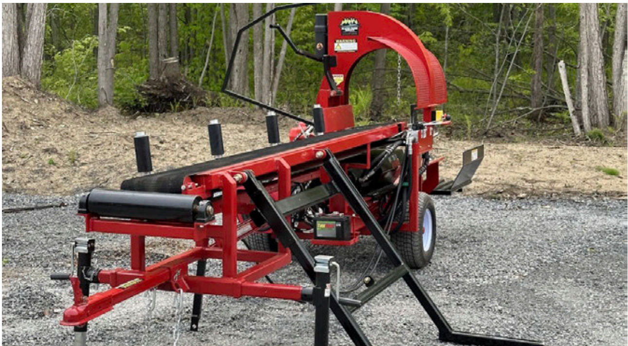
2000B-XL Processor is shown with optional Hydraulic Log Loader
